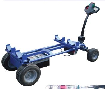
Originally designed to create a bespoke transport solution for a pipework installation project, this motorised trolley is ideal for securely moving heavy pipes and tubes around congested sites.
