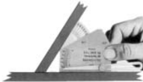
Checking Angle of Vertical Member
