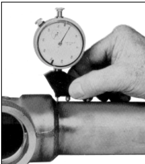
Measures Undercut Socket Weld
