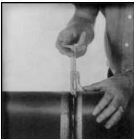
Measure internal mismatch, pipe wall.
