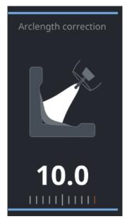
Example: Welding parameters for arc length correction -10 / 0 / +10  $\,$
