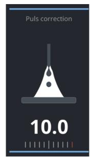
Example: Welding parameters for pulse correction -10 / 0 / +10
