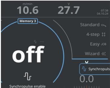
Example: Multifunctional button  ${\mathfrak Z}$  is assigned SynchroPulse, storage location "Memory  ${\mathfrak Z}$ "
