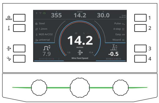
Control panel with welding screen for MIG/MAG
