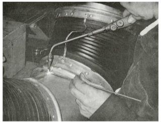
For repetition work other methods of pre-heating, such as air and gas torches etc, may be used. It is possible to speed up production by arranging procedures so that one or two assemblies are being pre-heated while others are being brazed.
