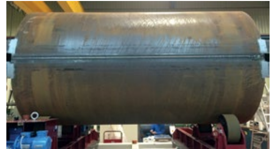
3m long 65mm thick welded in 11 minutes
