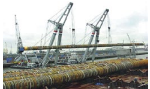
60m monopiles from 100mm plate
