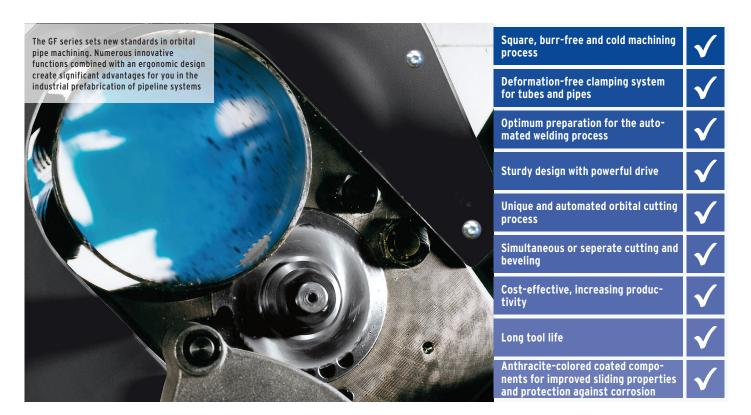
The basic requirement for the productive and high-quality welding of pipes with automated welding technology is a precise, right-angled and burrfree cut as well as a perfectly beveled pipe end. The GF series cuts and bevels high-alloy steel (stainless steel), low- and unalloyed steel, plastics, casting materials and non-ferrous metals easily and in just seconds, using the "Planetary Cutting" method. The powerful clamping is effected without any deformation of the workpiece.
