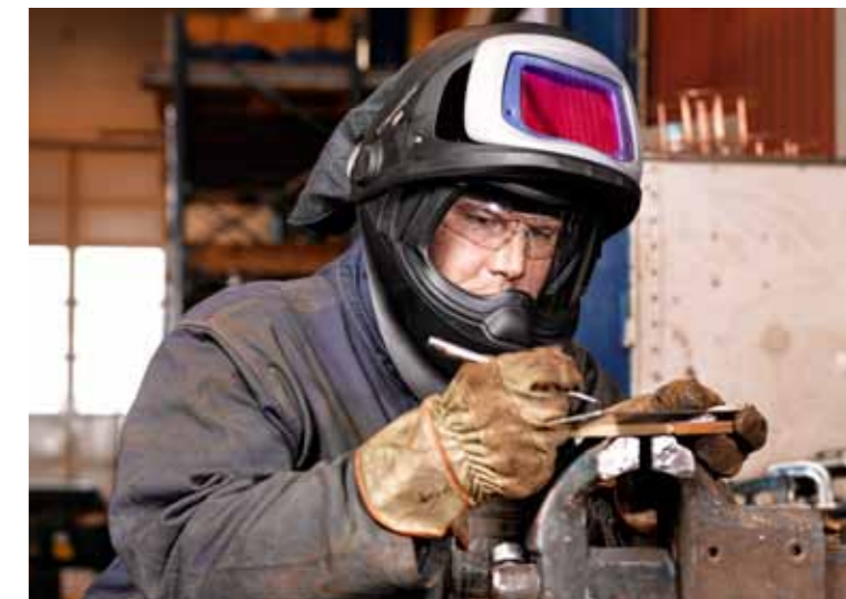
A quick lift of the silver front and you get a big, 17x10 cm, clear view — perfect for precision grinding in low light conditions, while maintaining respiratory protection.
