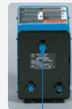
Auto ROI back panel showing connection for input and output signals.
