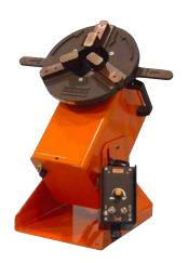
Table on the Gullco Model GP/GPP-200 Series of Welding Positioners (above left) is designed for mounting the WPG-250 Welding Gripper as indicated.
