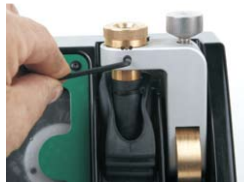
Three position grinding triples life of the wheel
